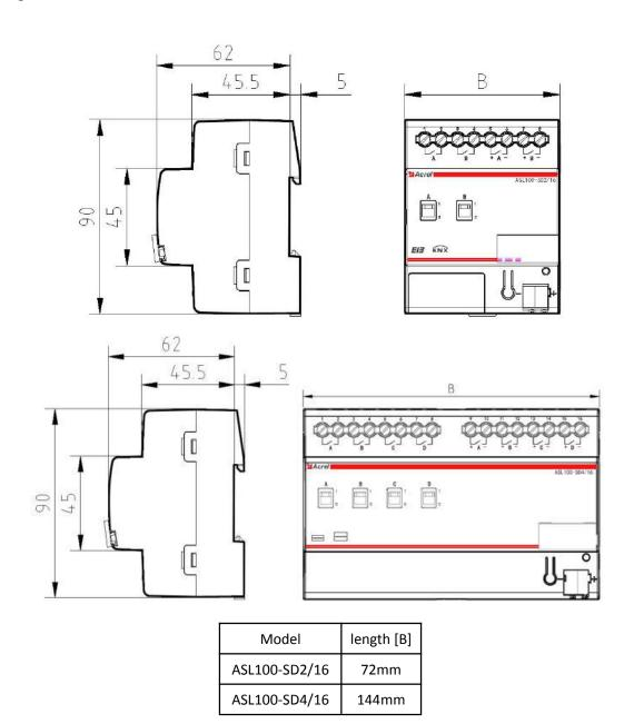
**Installation notes**: this module is applicable to 35mm track installation. You just need to clamp the module into the track for installation.
